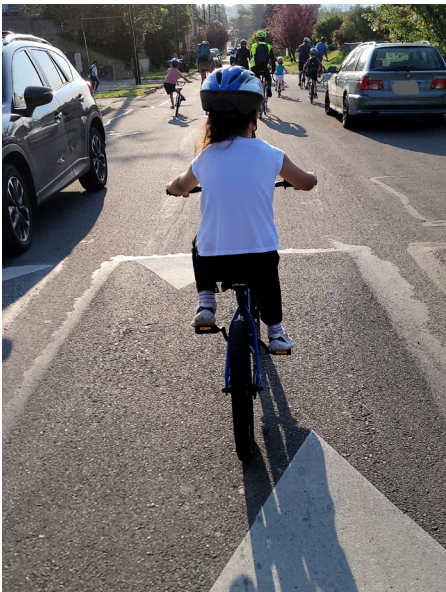
Speed cushions like the photo above are like speed humps but have a cut-out to better accommodate emergency vehicles. They're proven to slow down people driving.
